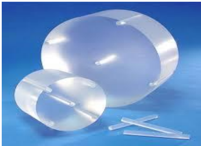
Figure 1: image of CT head phantom (small) and body phantom (large) [1]
