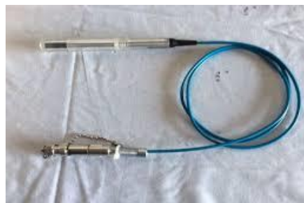
Figure 2: image of CT ion chamber [1]
