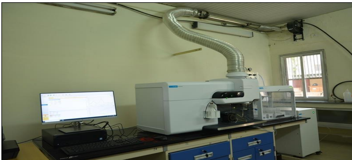
Plate 1: The Set-up of Agilent 4200 MP-AES
